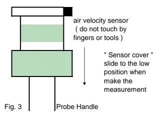
\* Do not use the fingers or any tools to touch the air velocity sensor, otherwise the meter may happen the permanent damage without warranty.
