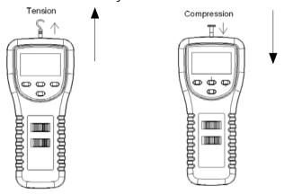
2) During the measurement, the SENSING HEAD along the adapter has to be on a line with measuring object. ( ref. Fig. 2 )
