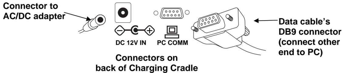
The QRAE II's cradle connects via a DB9 (9-pin) connector to a computer running ProRAE Remote software.
