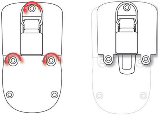
3. Hold the QRAE II down and lift the compartment cover by pulling on the belt clip.
