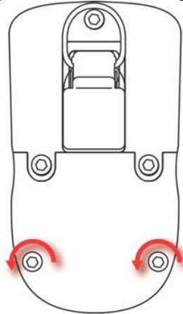
4. Push the screws from the back of the monitor to pop the cover off the front.
