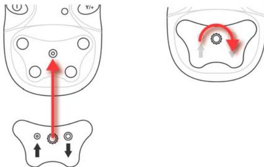
**Note:** Finger-tighten this only. Do not use a pliers or other tools. The Calibration Adapter should be snug, but an air-tight seal is unnecessary.
