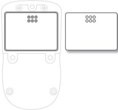
**Note:** Before installing the new battery, visually inspect the contacts to make sure they are clean. If they are not, wipe them with a soft cloth. Do not use solvents or cleaners.
