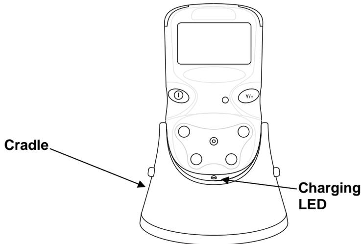
**Note:** Before setting the QRAE II into its charging cradle, visually inspect the contacts to make sure they are clean. If they are not, wipe them with a soft cloth. Do not use solvents or cleaners.
