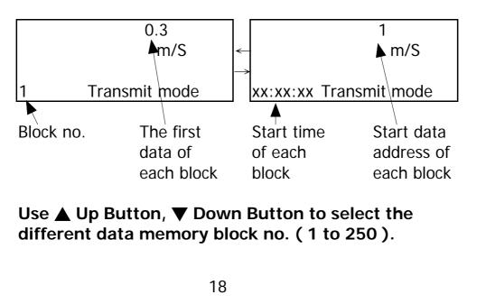
The meter can save 16,000 data max. , those data will saved into 250 memory block max.
