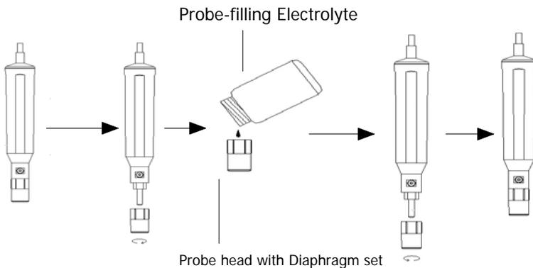
*The procedures that to fill the Probe's Electrolyte, refer the chapter 6-3 " Probe maintenance ", page 29 .*
