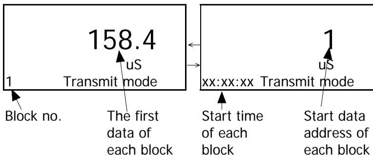
**Use "▲ Up Button", " ▼ Down Button " to select the different data memory block no. ( 1 to 250 ).**
