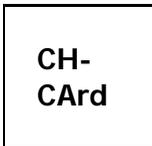
It means that the SD card exist the problem or the SD card memory is full, it should change SD memory card.
