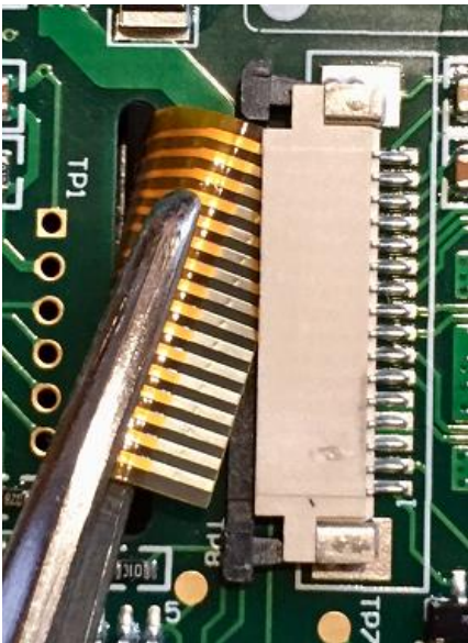
Using tweezers, carefully pull out the LCD cable band and remove the LCD.
