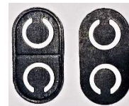
New gaskets are flat on both sides, but used ones develop grooves caused by the gasket sealing ridge. If re-using a gasket place the grooved side back facing the sealing ridge
