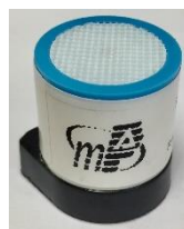
Single-Wing Low-power Sensor
