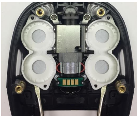
Pry off the left and right sensor cap assemblies
