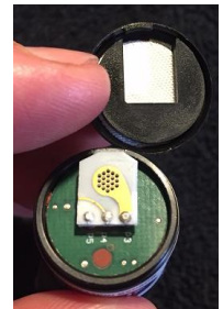
Alternate PID design 3-Pin sensor grid lamp alignment
