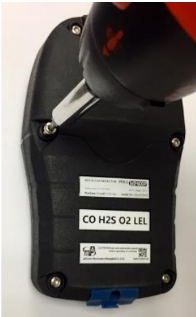
Remove the 6 housing screws (2-mm or 5/64" Allen wrench)
