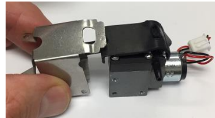
Pull the pump up and out (there is strong resistance and will need some rocking motion)
