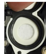
Sensor Gasket in Cap
