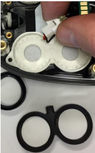
Remove the sensor gaskets and unplug the power connector
