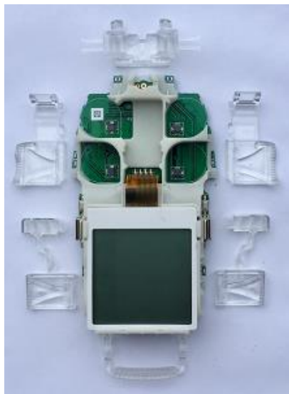
Pull off the alarm window/brackets
