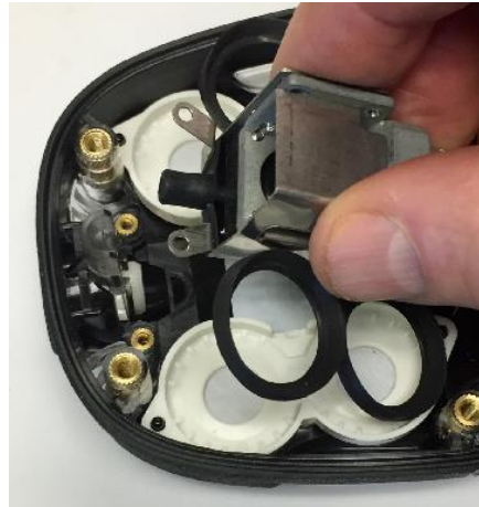
Pull the pump up and out (there is strong resistance and will need some rocking motion)
