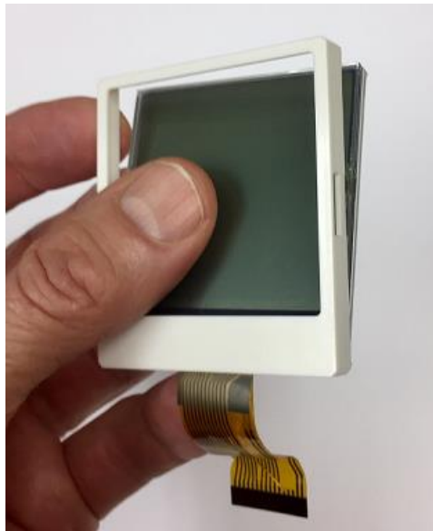
Push on the front of the LCD to remove it from the casing. Insert the new LCD, plug in the cable band, and reassemble the POLI.
