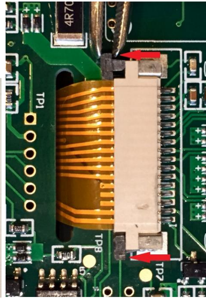
On the bottom of the circuit board, loosen the black retaining plugs that secure the LCD cable band.
